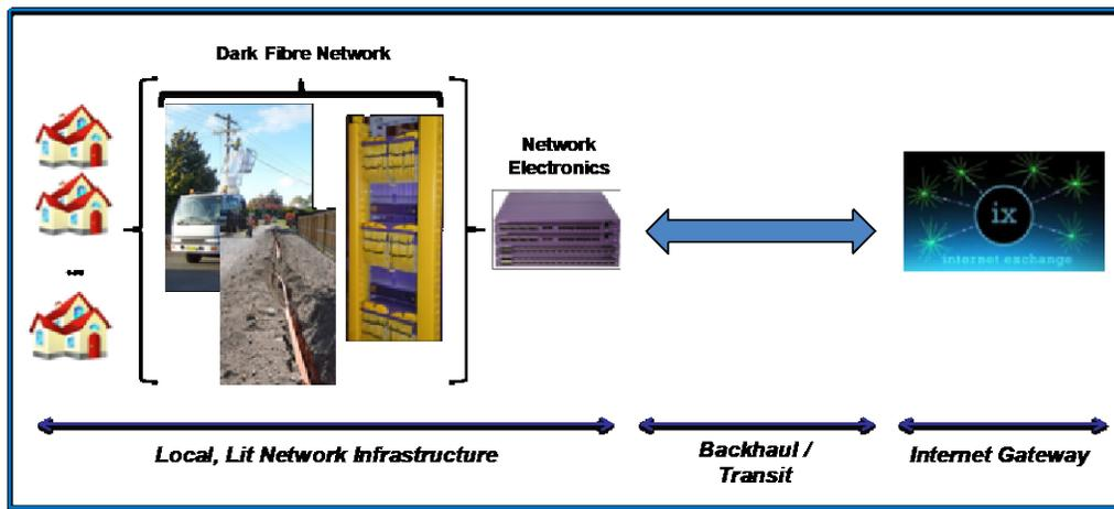
Figure 97. Local, Backhaul, and Gateway Components
