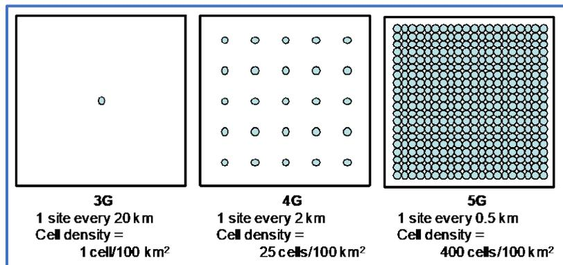
Figure 103. 5G Cell Tower Density Requirements
