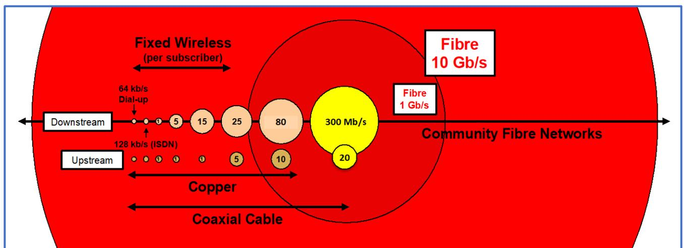
Figure 99. Connectivity Speed by Technology
