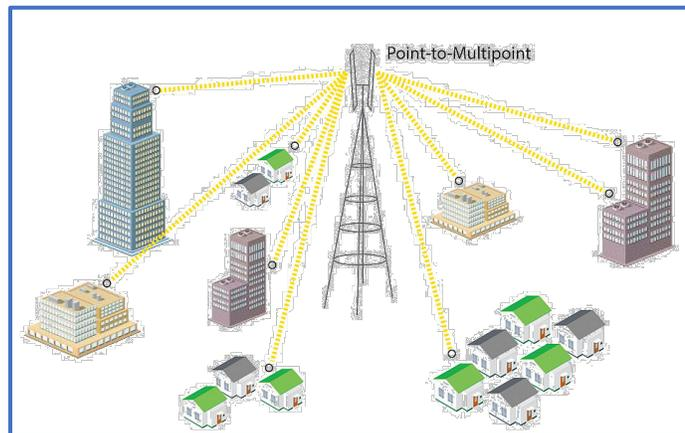
Figure 104. Point-To-Multipoint Fixed Wireless Networks
