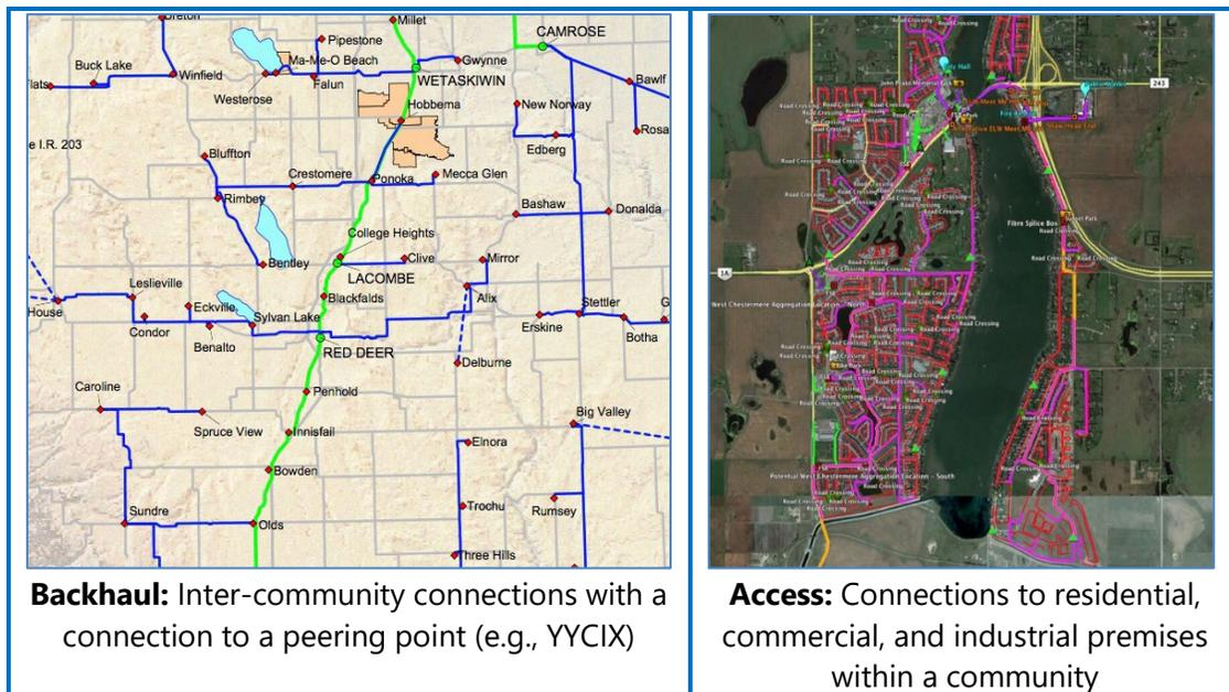
Figure 98. Backhaul Vs Access Networks – A Comparative View
